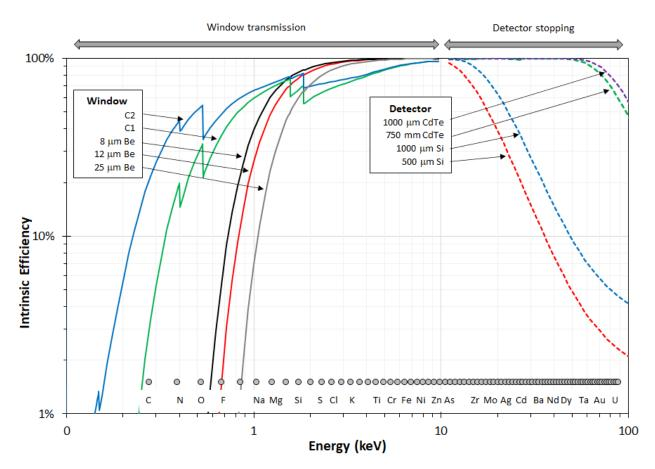
**Figure 4.** Comparison of the intrinsic efficiency of the X-123 detectors from Amptek. At low energies, the Be window limits sensitivity, and the 1 mm thick CdTe crystal (dashed violet curve) has a good efficiency up to 70 keV. © Amptek Inc 2021. Reprinted with permission.
