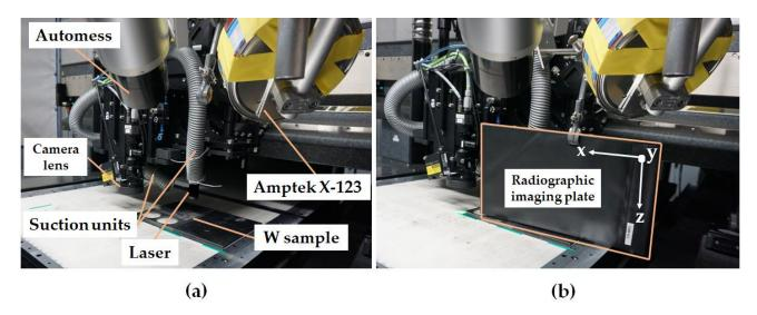
**Figure 3.** (a) Experimental setup and positioning of the measuring devices in the interior of the USP-laser machine. The Amptek X-123 spectrometer was placed in a tinplate box with an opening in front of the window and additionally covered with seven layers of 13 μm thick aluminum foil for shielding to prevent electromagnetic compatibility influences. (b) Placement of the radiographic imaging plate to detect the direction and homogeneity of the X-rays emission during USP-laser processing.
