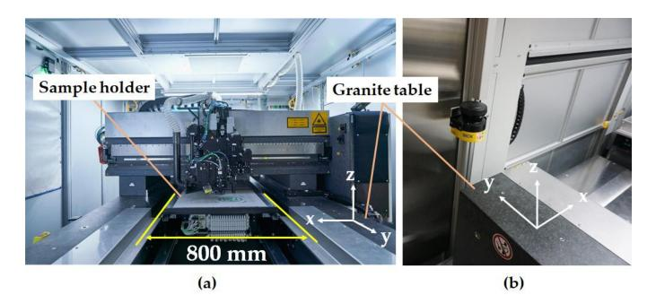
**Figure 1.** (a) Interior of the microSHAPE<sup>TM</sup> USP laser system at SCHOTT AG. The system is accessible and equipped with several safety systems that are intended to prevent staff from entering the machine during laser operation. One of these safety systems is the Sick laser scanner device (**b**) installed in the wall in front of the operating machine system. The monitored area covers the region between 10 cm and 30 cm above the granite table.
