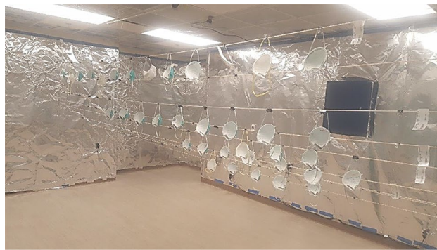
Figure 3. Picture taken of the sterilization room at hospital. The walls are covered with aluminum foil, and facemasks are strung on several different lines across the room.
