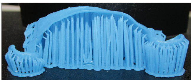
Figures 7: Three-dimensional printed castable framework
