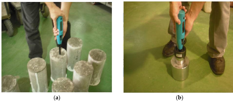
Figure 2. (a) Rebound hammer test; (b) rebound hammer calibration.
