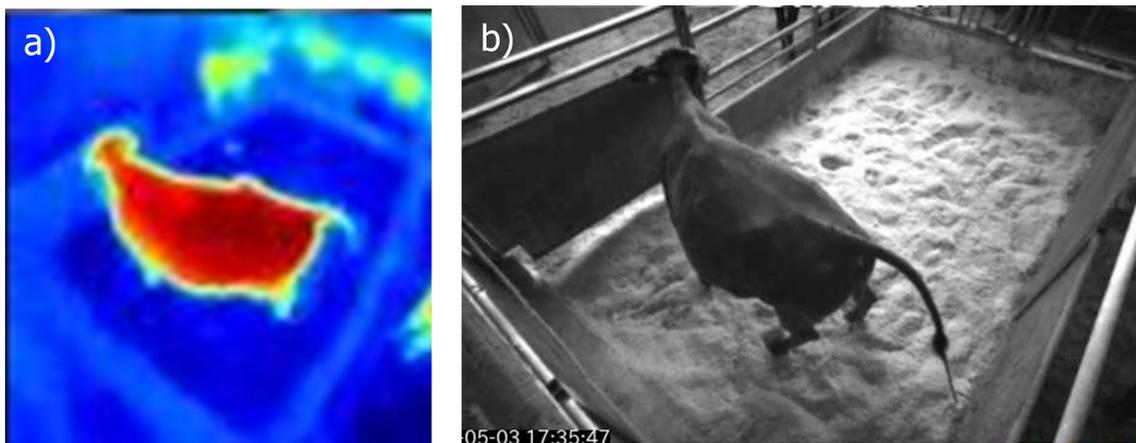
**Fig. 2.** Thermal (a) and visible (b) images obtained using the digital camera system. The distance moved was analyzed using thermal images (a), and postural change frequency and tail raising time were analyzed using visible images (b).
