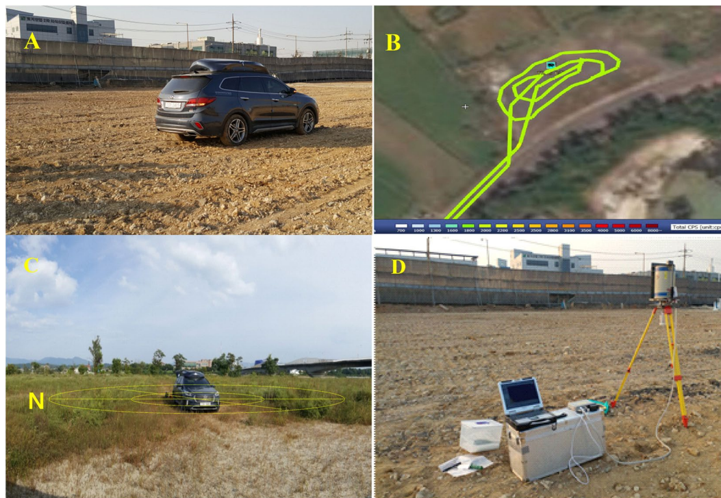
Figure 1. Pre-setting of gamma spectroscopic techniques of in-situ NaI(Tl) detector in the survey vehicle and in-situ HPGe detector. Colored line (B) represents the levels of total \gamma -ray count rate of NaI(Tl) detector automatically generated by the operating software (TRMS, Terrestrial \gamma -Radiation Monitoring System, made by RadSearch Co., Korea) of the car-borne measurement system on the satellite image of cesium ( http://cesiumjs.org ).
