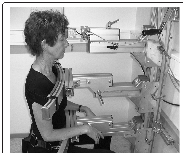
Figure 2 Cervico-thoracic flexion test. Sitting measurement of isometric cervico-thoracic flexion strength, maximal voluntary contraction (with permission).
