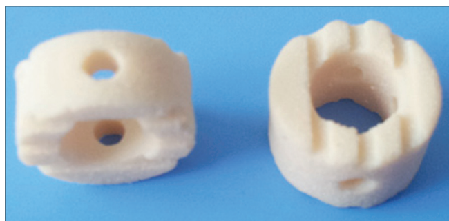
Figure 1: Photograph of hollow cylinder n-HA/PA66 cage. Each cage has wide rims with several shallow recesses designed to prevent subsidence and migration
