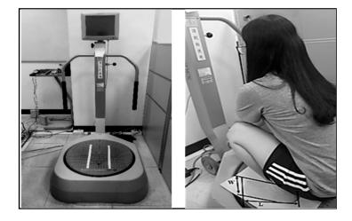
Figure 2. Measurement of squatting stability on the Biodex balance system platform.
