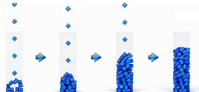
**Figure 12.** Dynamics of packing process for packing of cylinders with  $\text{COR} = 0.9$  and  $\mu_d = 0.1$  in a tube with  $N = 4.69$ . A video of a packing process with  $\text{COR} = 0.1$  and  $\mu_d = 0.9$  with  $N = 5$  is supplied in the Supporting Information.
