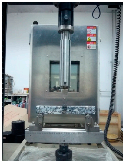
Figure 8. Low temperature bending test process.
