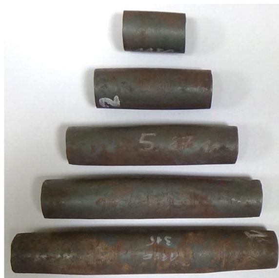
Figure 8. The samples deformed in the rotational compression of bars; respectively, from the top, the samples formed from billet with the length equal 30, 60, 90, 120 and 150 mm.
