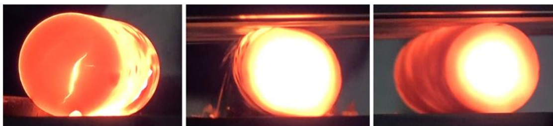
Figure 3. Rotational compression of a sample with the initial length equal 90 mm with the reduction ratio 1.15; the temperature of the billet 1150 °C.
