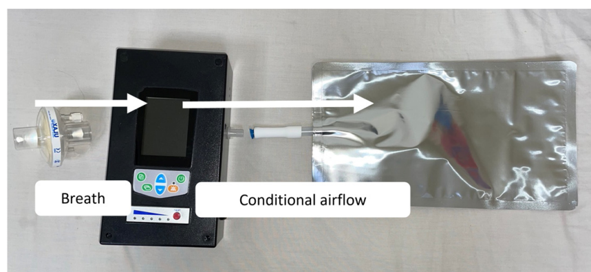
Figure 2. Exhaled breath sampling design. We used disposable single-use mouthpieces (bacterial/viral filter with HME, Ab ULAX, Motala, Sweden) and disposable single-use sampling bags (1000 mL aluminized gas collection bag, Hope Wang Enterprises, Taipei, Taiwan). In order to collect endogenous VOCs, we used a specific collector device that was developed by Professor Yao-Kun Li's laboratory in the Department of Applied Chemistry at National Yang Ming Chiao Tung University. As the concentration of carbon dioxide reached the level that equates to alveoli air, the collector device began directing exhaled breath to flow into the air sampling bag connected to it at a fixed flow rate. The red flashing light on the device indicated that the directing process had started, allowing both the sampling personnel and the subject to confirm proper collection.
