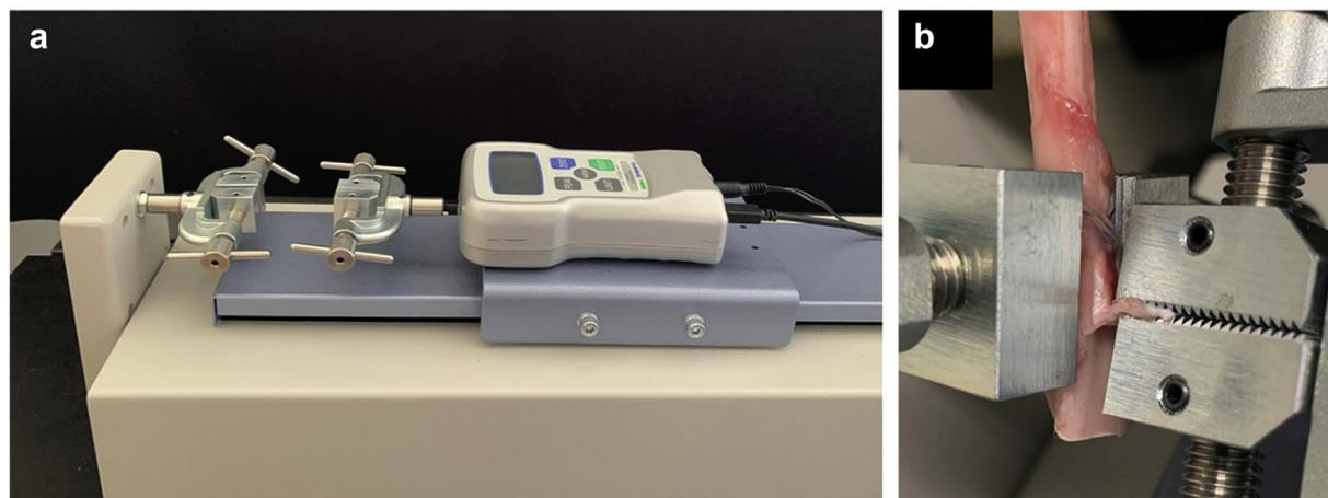
**Figure 3** Biomechanical test setting. (a) A (right) holding device is connected to a digital force measuring instrument. (b) A (left) holding device is grasping a tibial bone, and a (right) holding device is grasping a tendon graft.
