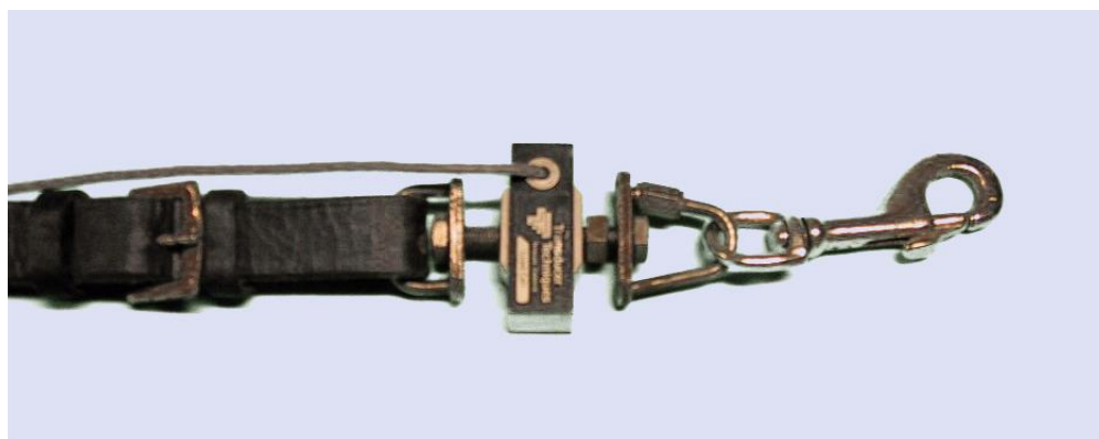
Figure 5. Strain gauge attached securely to the rein (left) with a metal clip for attachment to the bit. Note that none of the components are elastic. (image from [5]).
