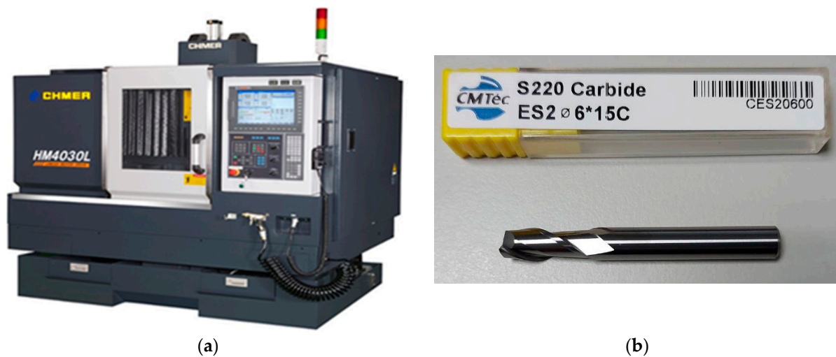
Figure 1. Experiment setup. (a) Three-axis CNC machine tool (HM4030L). (b) Tungsten carbide end milling cutters with 2 blades and no coating.
