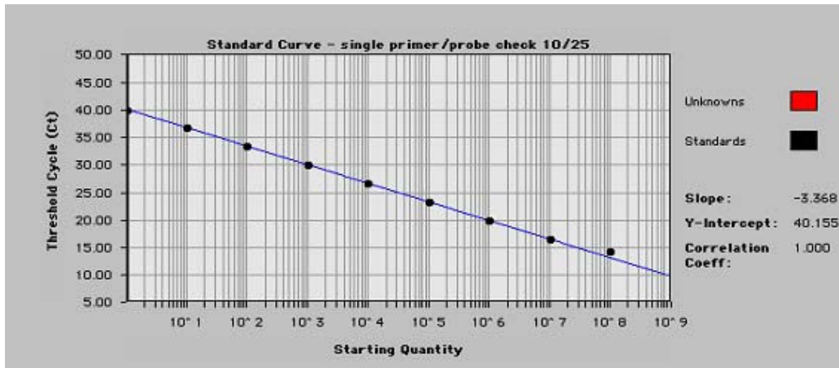
Figure 5 IFN \gamma real time RT-PCR standard curve (linearity). Linear response (IFN \gamma plasmid copy number vs. Ct) is shown. Curve characteristics are also indicated.
