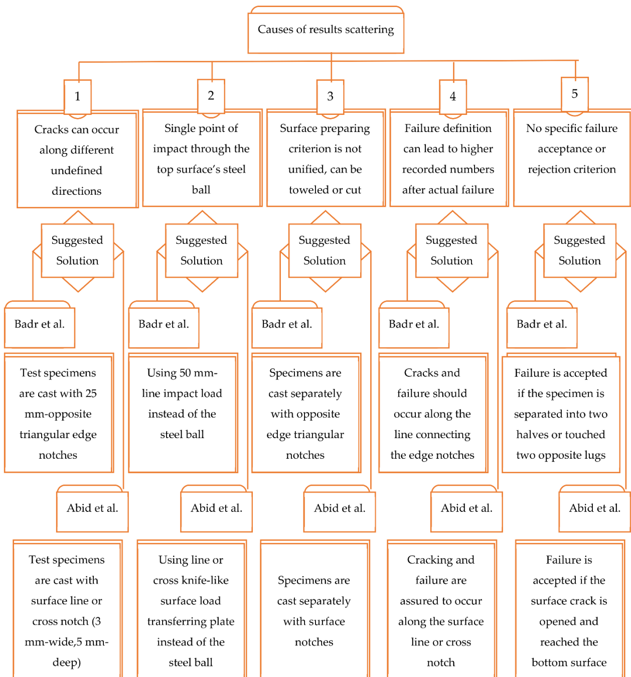
Figure 12. Sources of ACI 544-2R repeated impact scattering of results and suggested modifications by previous studies.
