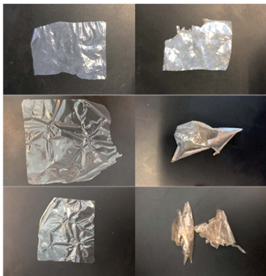
Fig. 6 Photographs of the L-AEM samples before (left) and after (right) immersion in aqueous KOH ( 1 \text{ mol dm}^{-3} ) at 80 \text{ }^\circ\text{C} for 1000 h: (top row) L-AEM-TMA, (middle row) L-AEM-MPY, and (bottom row) L-AEM-MPIP.
