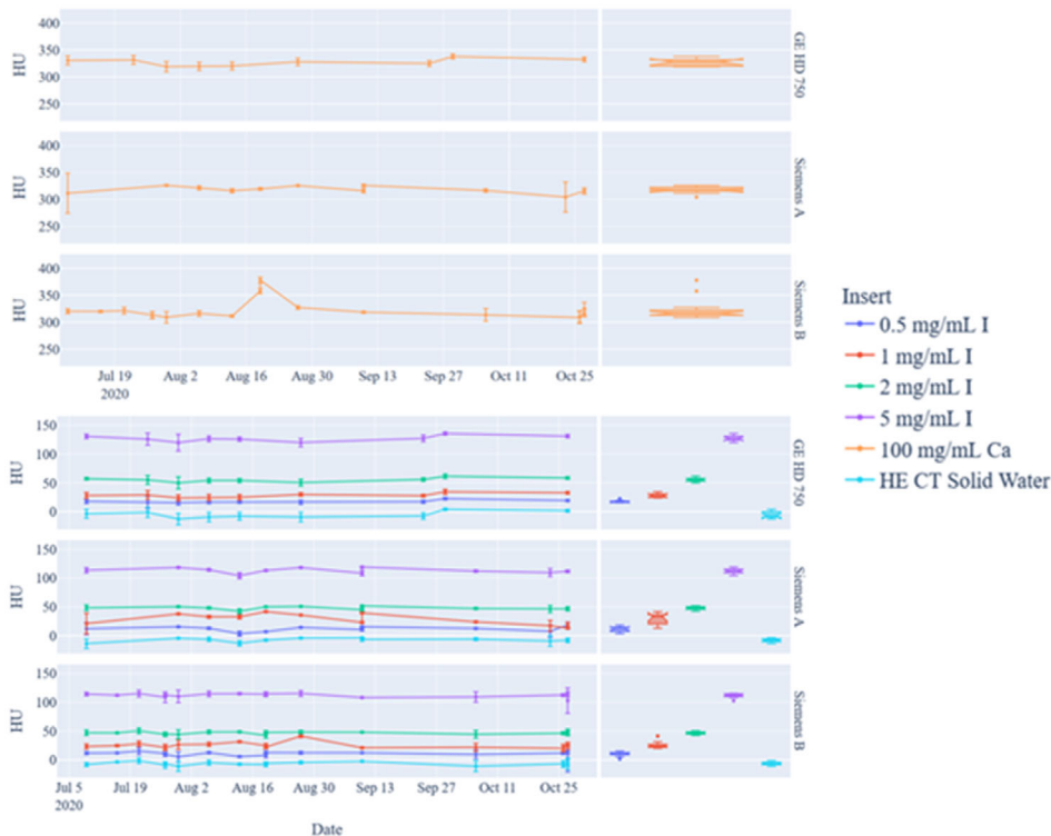
FIGURE 4 Dual-energy quality control (DEQC) analysis of the dual-energy computed tomography (DECT) phantom for blended dual energy images based on phantom inserts (top) calcium-insert only (bottom) iodine inserts and solid water background (left) scatterplot showing mean HU and standard deviation values for each insert over a 3-month period for the specified phantom inserts (right) box plot of measured values
