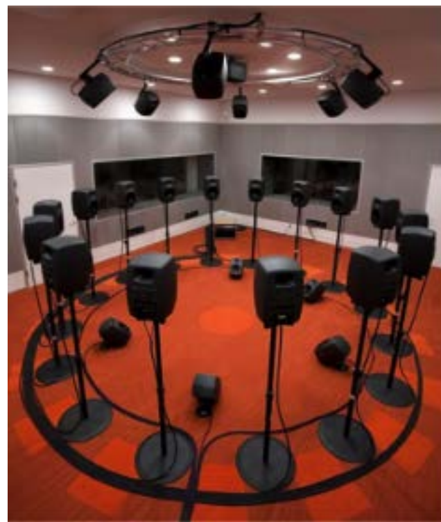
Figure 1. Physical test setup used for the measurements. Only the 16 loudspeakers in the horizontal plane were used in the current study.
