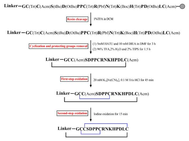
Figure 2. Schematic of the synthetic route for cyclic analogues of  $\alpha$ -conotoxin TxIB.
