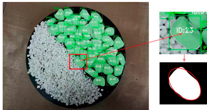
Figure 5. Ellipse fitting method. This method can fit masks after segmentation into ellipses and support the subsequent measurement of rotation angles.
