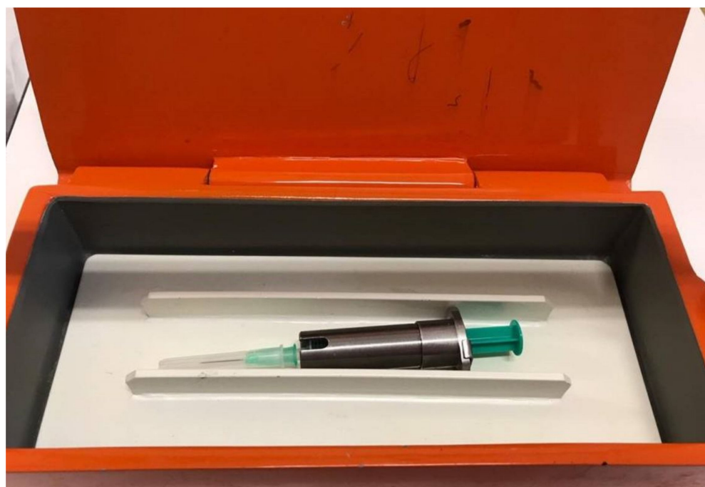
Figure 1. Shielded syringe with radioisotope (2 mL of ^{111}\text{In-DTPA} ).
