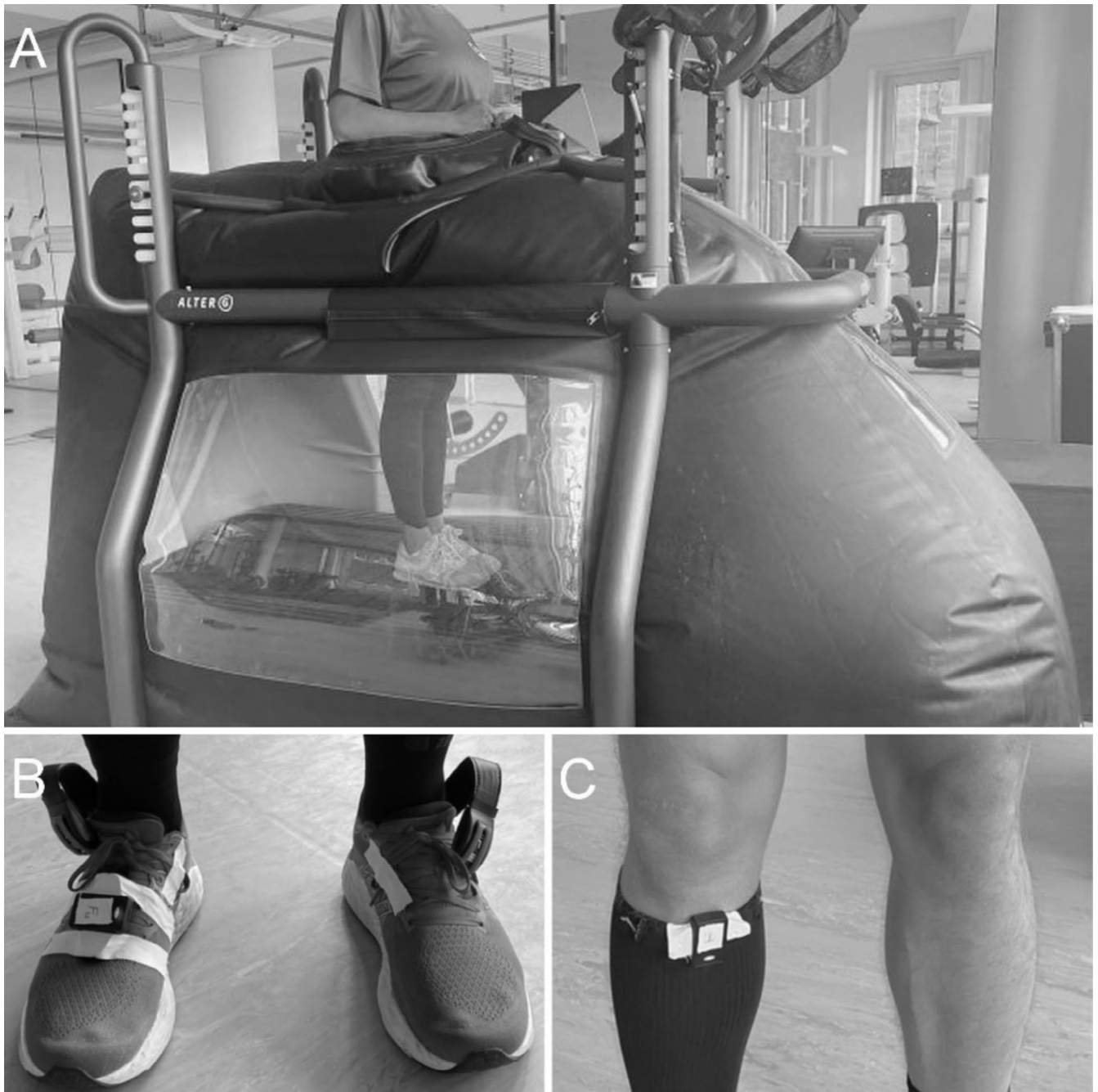
FIGURE 1 | Instruments used in this study. (A) lower body positive pressure treadmill (LBPPT), fully inflated. The air chamber is attached to the bars around the athlete's waist where it is zipped to the neoprene skirt. (B) In-shoe pressure measuring soles and foot inertia sensor. The soles corresponding data logger was attached to the lacing. The IMU was attached in the front of the lacing with push buttons. (C) Tibial inertia sensor. The IMU was attached to an elastic calf sleeve with push buttons and positioned to the medial proximal part of the tibia.
