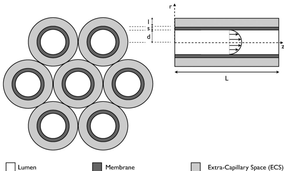
**Figure 1.** A schematic of the HFB setup. The left-hand schematic shows the structure of a fiber bundle, comprising seven Krogh cylinder units. The right-hand schematic shows a cross-section through an individual fiber, including the fluid velocity profile in the lumen.
