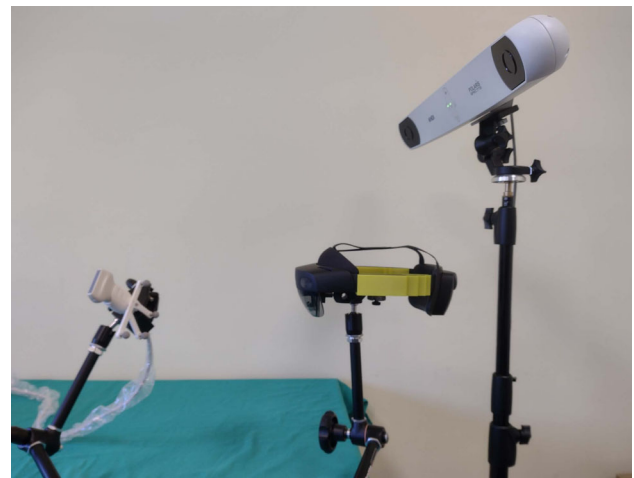
Fig. 4 Setup for the static tracking accuracy evaluation. HoloLens 2 and the OTS are fixed, while the US probe with its marker is moved to 20 different poses for measurement acquisition
