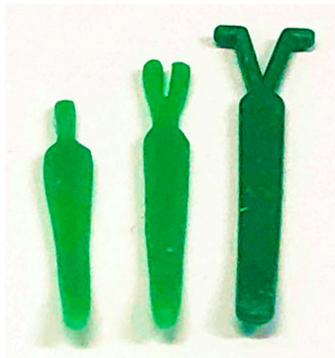
Figure 2. Kobayashi plug: Initial type (left), Prototype (middle), New type (right).
