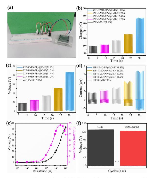
**Figure 10.** (a) Photograph of C-TENG, (b) transfer charge, (c) open-circuit voltage and (d) short-circuit current of C-TENG, (e) power output of C-TENG on external load resistances, (f) stability test of the C-TENG.
