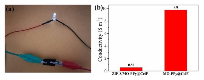
**Figure 8.** (a) Lighting of an LED using the ZIF-8/MO-PPy@CelF with 31.8% ZIF-8 deposition ratio (0.85 mm thick); (b) Conductivity values of ZIF-8/MO-PPy@CelF and MO-PPy@CelF.
