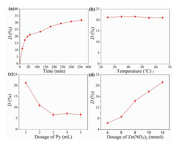
**Figure 2.** Effect of time (**a**), temperature (**b**), dosages of Py (**c**) and Zn(NO<sub>3</sub>)<sub>2</sub> (**d**) on ZIF-8 deposition. Process conditions: (**a**) 25 °C, Py 1 mL, Zn(NO<sub>3</sub>)<sub>2</sub> 12 mmol; (**b**) Py 1 mL, Zn(NO<sub>3</sub>)<sub>2</sub> 12 mmol, 1 h; (**c**) 25 °C, Zn(NO<sub>3</sub>)<sub>2</sub> 12 mmol, 1 h; (**d**) 25 °C, Py 1 mL, 1 h.
