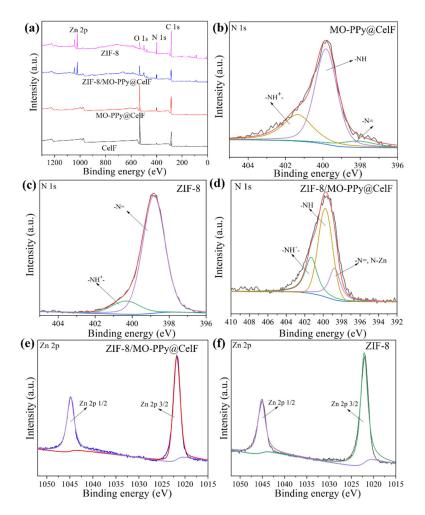
**Figure 6.** (a) XPS wide scan spectra of CelF, MO-PPy@CelF, ZIF-8 and ZIF-8/MO-PPy@CelF; (b–d) N 1s XPS spectra of MO-PPy@CelF, ZIF-8 and ZIF-8/MO-PPy@CelF; (e,f) Zn 2p spectra of ZIF-8/MO-PPy@CelF and ZIF-8.
