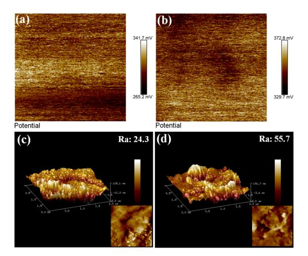
**Figure 9.** Surface potentials of ZIF-8/MO-PPy@CelF with 17.4% (**a**) and 31.8% (**b**) ZIF-8 deposition ratios; Surface roughness values of ZIF-8/MO-PPy@CelF with 17.4% (**c**) and 31.8% (**d**) ZIF-8 deposition ratios.
