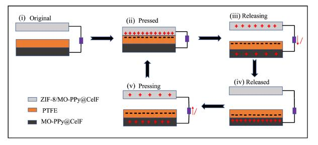
Figure 7. Schematic illustration of the TENG working principle.
