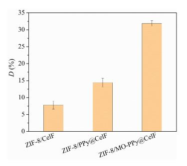
**Figure 1.** Comparison of ZIF-8 growth on three CelF substrates. Process conditions: 25 °C, Py 1 mL, Zn(NO<sub>3</sub>)<sub>2</sub> 12 mmol, 6 h.
