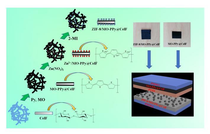
Scheme 1. Schematic illustration of preparation and application of ZIF-8/MO-PPy@CelF composite.
