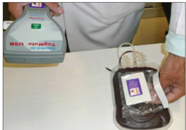
Figure 2: Standard temperature monitoring system and its reader
