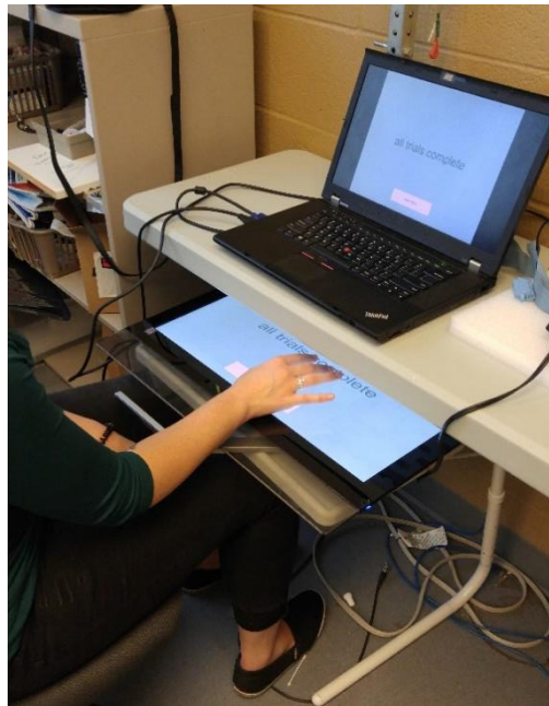
Figure 2. Motor skill acquisition tracing task setup. A laptop is placed on the table, displaying the motor training task. A large touchscreen is placed on a desk directly below the table, ensuring that the table blocks the participants' view of their own arm. To control the sweep of each sinusoidal wave, participants were required to adjust to the velocity and amplitude of the traces by performing internal and external rotation of the right shoulder joint.
