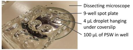
**Figure 5.** The setup for imaging and/or direct observation of regeneration with an upright microscope. In each 4 µL droplet hanging from the coverslip, there is one cell undergoing regeneration. Water in the wells of the glass spot plate limits evaporation of the droplets. This setup allows following the regeneration of multiple cells in parallel. Please click here to view a larger version of this figure.
