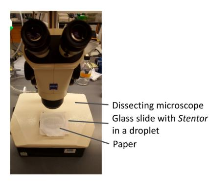
**Figure 2.** *Stentor* **cutting set-up.** Cell cutting is performed by manually manipulating a glass needle while looking at the cell using a commercially available dissecting stereo microscope. The purpose of the tissue paper is to provide the white background to see the cells better. Please click here to view a larger version of this figure.
