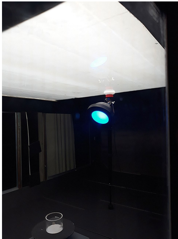
Figure 1. Wind tunnel setting of LED testing. The roof light (white top) is prevented from reflecting light on the glass plate of the cone (yellow LED shining through the glass plate) by facing 45° downwards.
