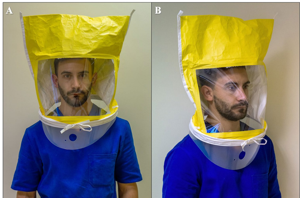
Fig. 2 The 3M™ Qualitative Hood Test Apparatus (3M, St. Paul, MN, USA) in frontal (A) and right oblique (B) views
