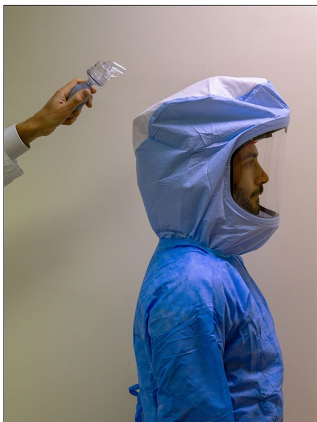
Fig. 4 A right profile view of the 3M™ FT-10 Fit Test (3M, St. Paul, MN, USA) using the ViVi® (THI, Total Healthcare Innovation GmbH, Feistritz im Rosental, Austria) SSHS: solutions were nebulized 10 to 15 cm from the inflow filter system
