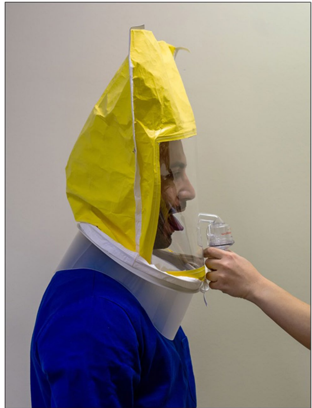
Fig. 3 A right profile view of the sensitivity test performed using the 3M™ FT-10 Sensitivity Test Kit (3M, St. Paul, MN, USA) and throughout any puffs of a sodium saccharin solution administered through a hole made in the anterior part of the visor of the 3M™ Qualitative Hood Test Apparatus (3M, St. Paul, MN, USA)
