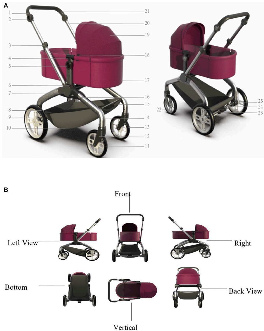
FIGURE 1 (A) Novel design of the baby stroller. 1. Handle rotation connection device; 2. Rotation button; 3. Pull button; 4. Sleeping basket fixing part; 5. Sleeping basket rotation button; 6. Handle rotation button; 7. Middle connector; 8. Rear wheel outer ring; 9. Rear wheel rim; 10. Storage basket; 11. Front wheel rim; 12. Front fork; 13. Front wheel outer ring; 14. Front foot tube; 15. Storage basket; 16. Aluminum strip; 17. Sleeping basket; 18. Awning fixing buckle; 19. Awning; 20. Aluminum tube; 21. Handle; 22. Brake pedal; 23. Brake control device; 24. Brake pipe; 25. Rear wheel fixing pipe; 26. Rear wheel fixing pipe. (B) Six views of the baby stroller.
