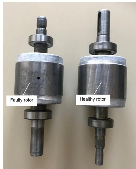
Figure 3. Healthy and faulty rotors.
