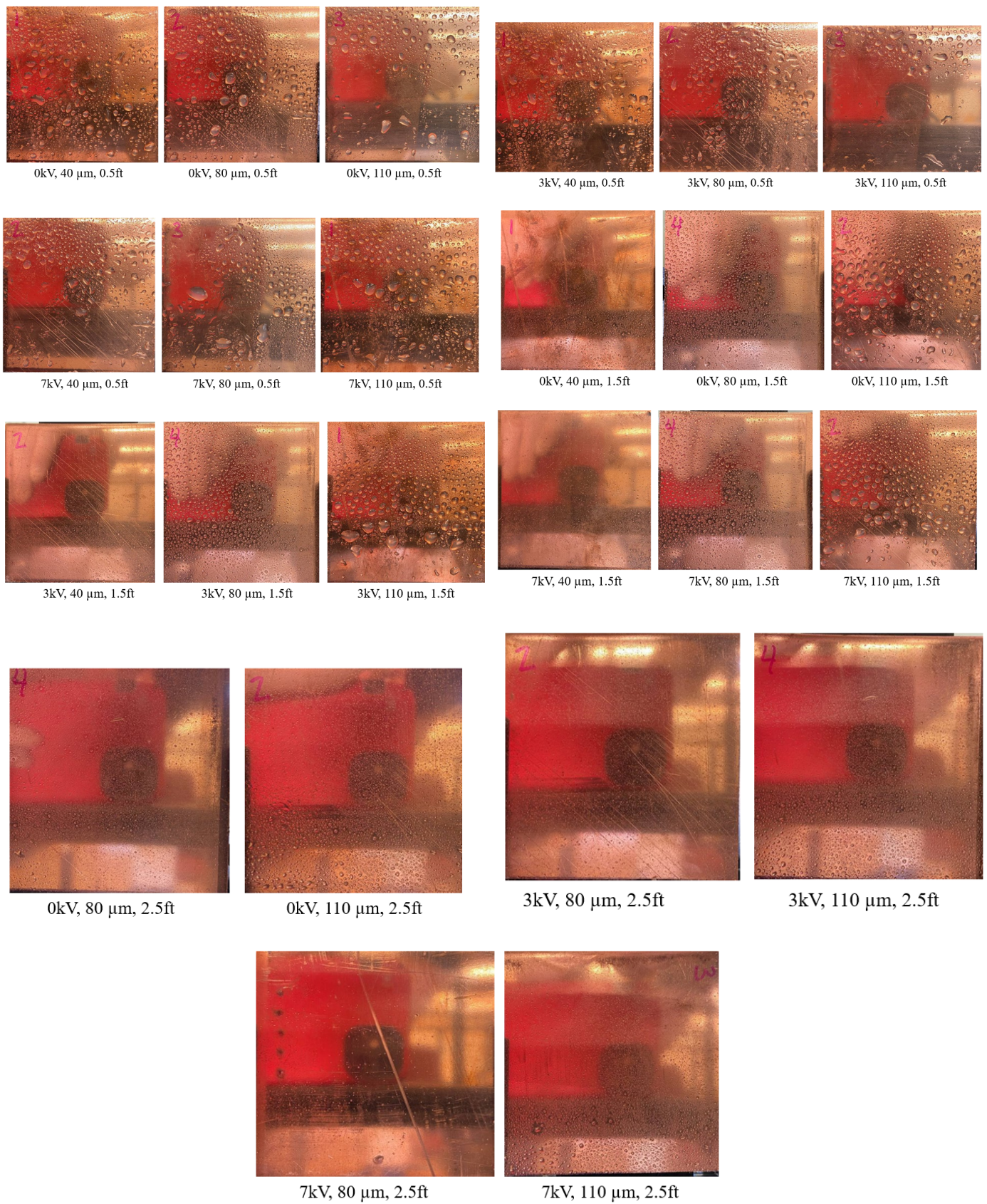
Figure A11. Copper: qualitative images of electrostatic deposition under various system parameters.
