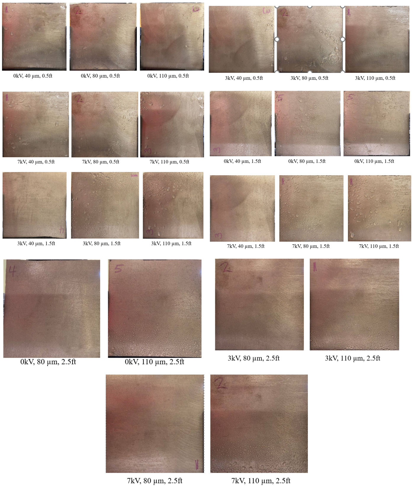
Figure A15. Stainless steel: qualitative images of electrostatic deposition at various system parameters.
