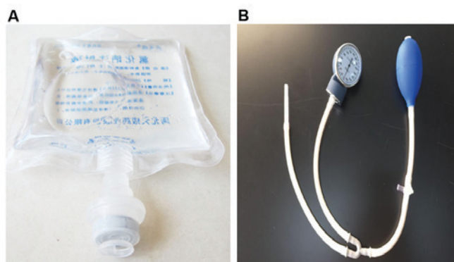
Figure 1. Pressure treatment of cells. (A) A normal saline bag was used to contain the culture dish. (B) Sphygmomanometer. Cells ( 1 \times 10^5 ) were plated in a 3.5 cm culture dish 1 day prior to experiments. The bottom of a bag containing normal saline was cut open with scissors and the contents was poured out. The culture dish was placed into the empty bag, and the bottom was sealed with a plastic-envelope machine. A pressure instrument was utilized to pump air into the bag, and the pressure was measured using the instrument. Cells in the different experimental groups were treated with various pressures using this method.
