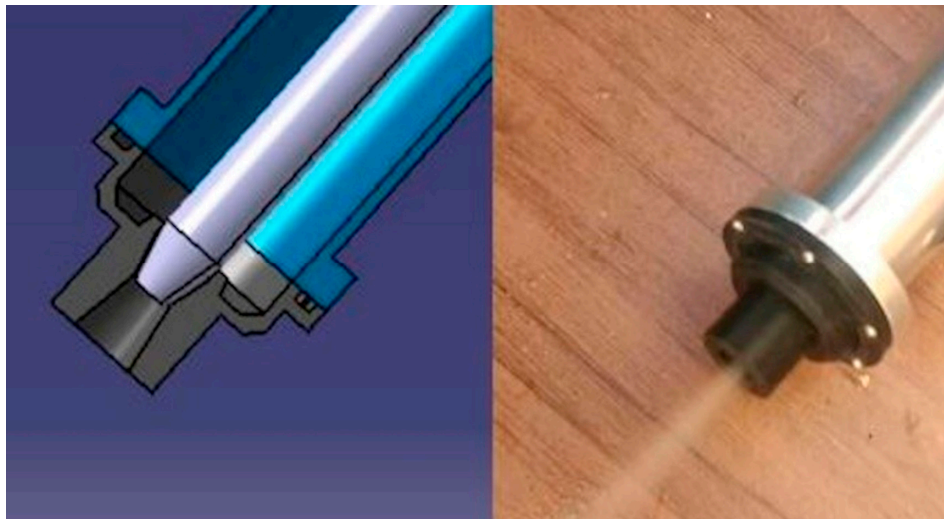
Figure 6. CAD design and the assembled valve.
