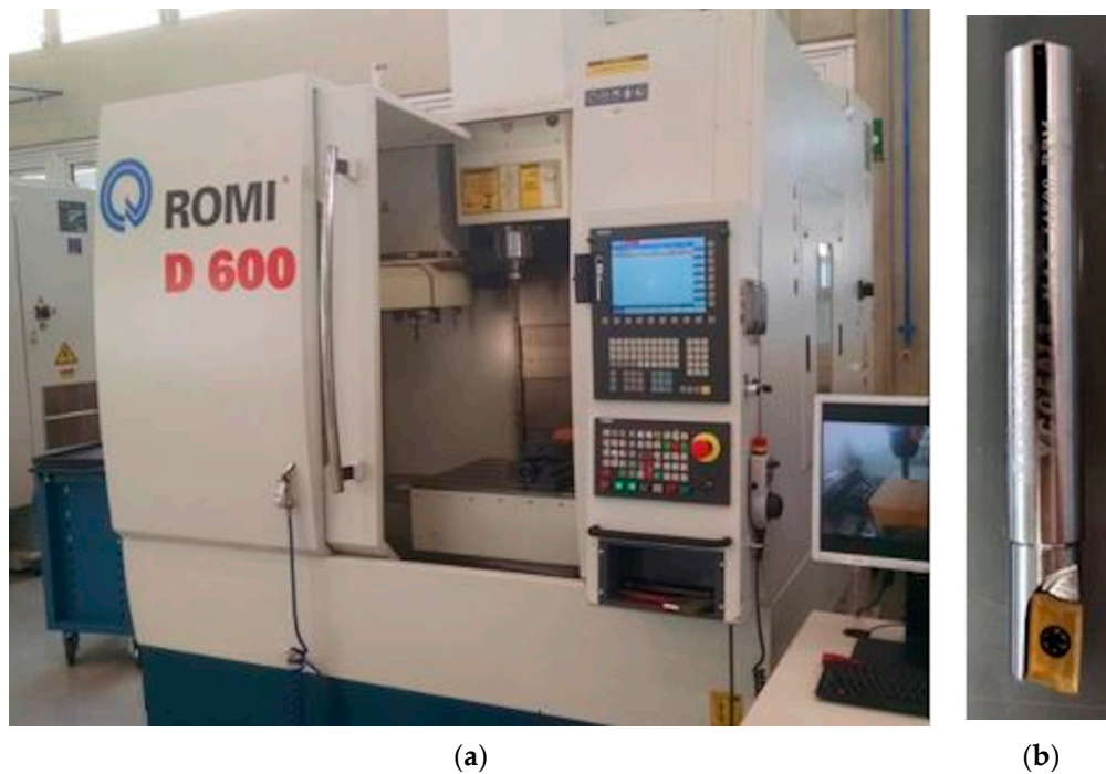
Figure 3. (a) ROMI D600 machining center and (b) KYOCERA tool used for milling.
