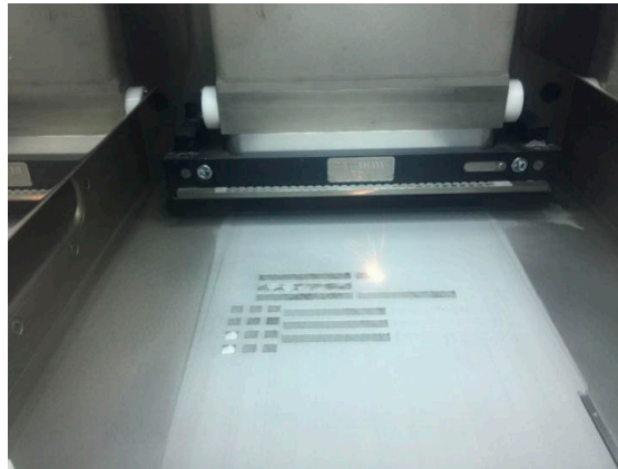
Figure 2. Selective laser melting of the cobalt-chromium alloy molding process.
