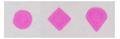
Figure 5. Stencil printed discs of 3 geometries using ink formulation HPMC 16% (500 µm stencil height).
