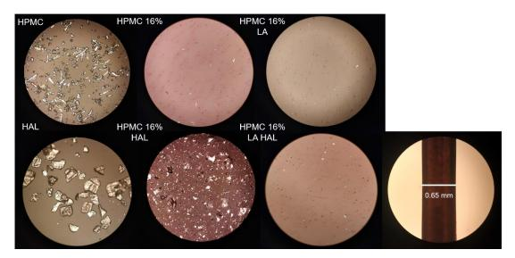
**Figure 8.** Polarized light microscopy of raw materials HPMC and haloperidol (HAL) and printed discs HPMC 16%, HPMC 16% lactic acid (LA), HPMC 16% LA HAL, and HPMC 16% HAL (magnification  $\times$ 10), stencil height 500 µm.
