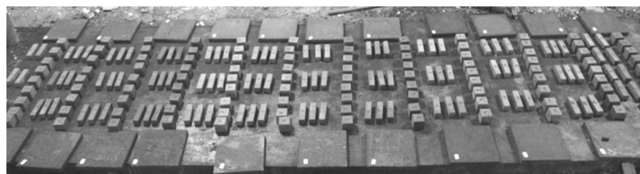
Fig 1. Image of the specimens after demolding.
