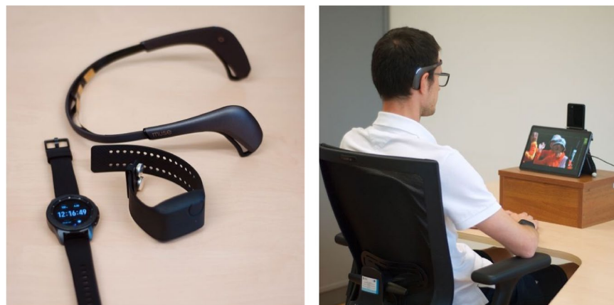
Fig. 2 Devices used to gather the physiological data and the experimental stand.
