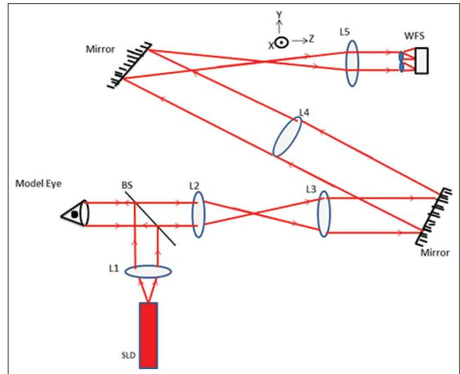
Figure 1: Experimental setup of a Shack-Hartmann Wavefront Sensor
