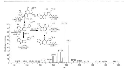
Figure 8. MS/MS Spectra and fragmentation pathway of degraded product with 309.33 m/z.
