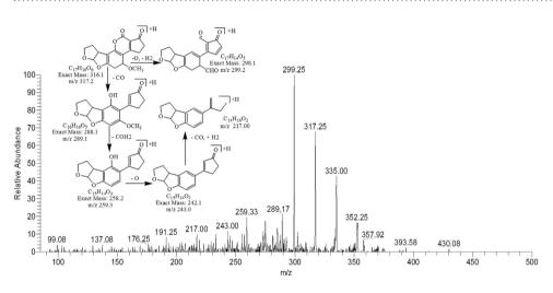
Figure 12. MS/MS spectra and fragmentation pathway of degradation product with 317.25 m/z.
