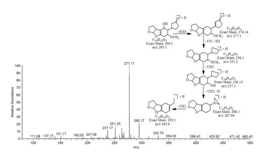
Figure 5. MS/MS Spectra and fragmentation pathway of degraded product with 295.17 m/z.
