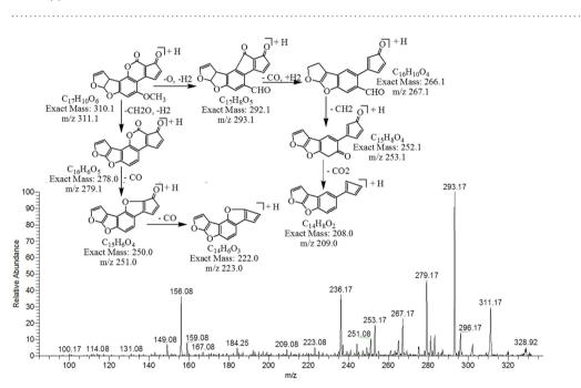
Figure 3. MS/MS Spectra and fragmentation pathway of degraded product with 311.17 m/z.
