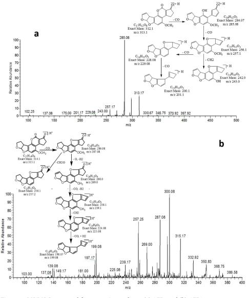
Figure 1. MS/MS Spectra and fragmentation pathway. (a) AFB1 and (b) AFB2.
