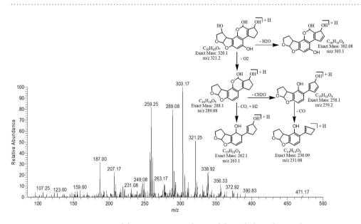
Figure 10. MS/MS Spectra and fragmentation pathway of degraded product with 321.25 m/z.
