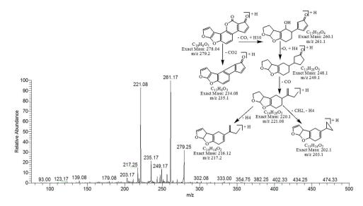
Figure 4. MS/MS Spectra and fragmentation pathway of degraded product with 279.25 m/z.
