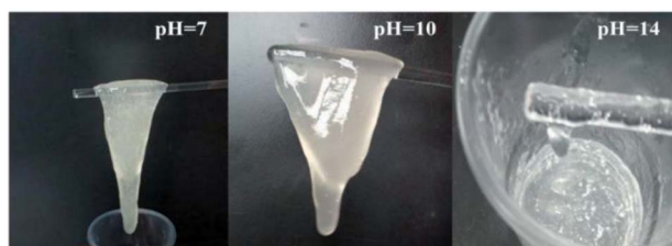
Fig. 8 Effect of pH on the hanging performance of NBC crosslinked fracturing fluid.
