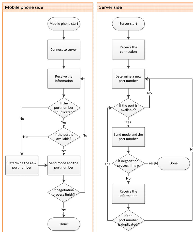
Figure 5. Smartphone- and server-based port negotiation processes.
