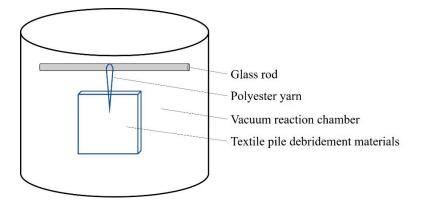
Figure 1. Illustration of the plasma treatment setup.
