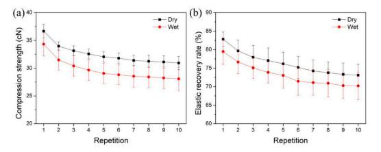
**Figure 9.** Influence of repetition on (**a**) compression strength and (**b**) elastic recovery rate of textile pile debridement materials in dry and wet states.
