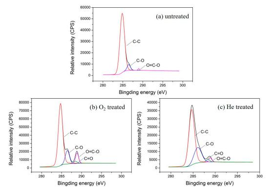
Figure 7. C1s spectra of the (a) untreated, (b) oxygen, and (c) helium plasma-treated textile pile materials.
