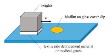
Figure 3. Experiment setup of the in vitro removal of biofilm.
