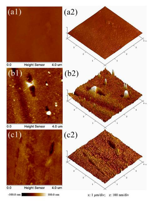
**Figure 5.** AFM images of polyester fiber surface (**a**) before and after (**b**) oxygen and (**c**) helium plasma treatments.
