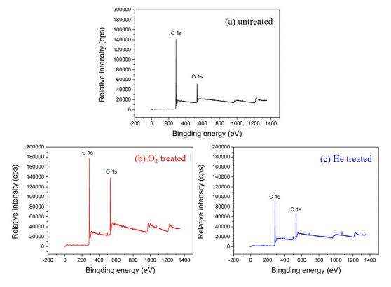
**Figure 6.** XPS overall scans of the (**a**) untreated, (**b**) oxygen, and (**c**) helium plasma-treated textile pile materials.
