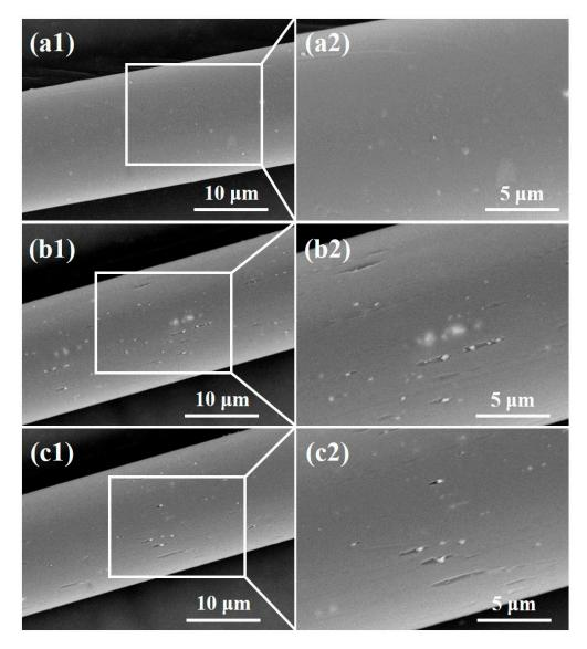
**Figure 4.** SEM images of the polyester fiber surface (**a**) before and after (**b**) oxygen, (**c**) helium plasma treatments.
