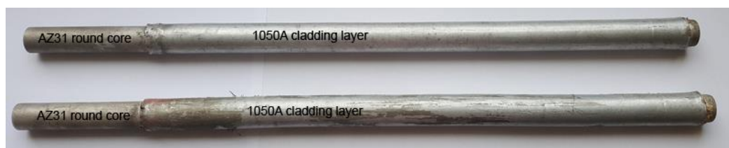
Figure 1. View of round Mg/Al bimetallic feedstocks after explosive welding.
