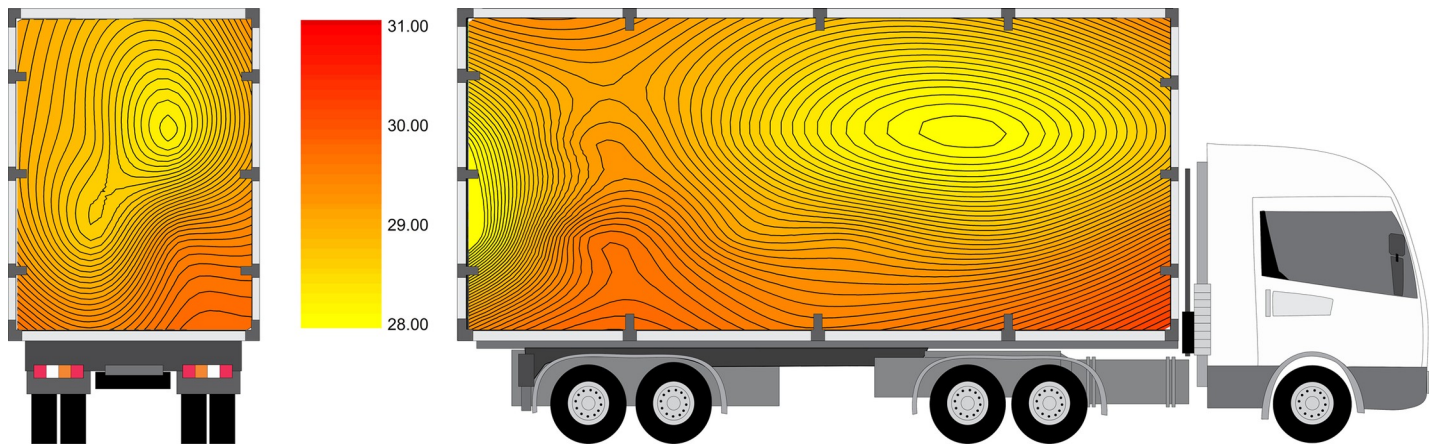
Fig 3. Mean temperature inside the crates ( T_{\text{crate}} ) in rear-to-front and lateral views. The truck is only for illustrative purposes.
